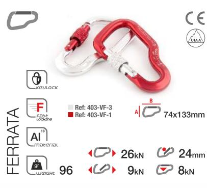
Carabiner with big opening made of aluminium and designed for Via Ferrata. Automatic fast lock facilitates handling and ergonomic geometry ensures a good grip. It has keylock lock and is anodized in red and silver
